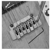
**Correctly-adjusted bridge** In the picture above you can see the typical saddle arrangement of an electric guitar with "normal" action after the intonation was correctly set.
