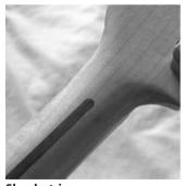
**Skunk stripe** The cover strip fitted over a truss rod installed from the back is often made from contrasting wood. That's why it was given its graphic name after the skin pattern of an animal called skunk.
