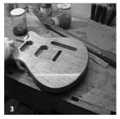
easy to apply: two to three coats are totally sufficient; allow each coat to dry for several hours. Instead of buying Danish Oil you can make your own by mixing one part of varnish, one part of boiled linseed oil and one part of mineral spirits. It's always a good idea to pour everything through a paint strainer to remove impurities and undissolved residue.
