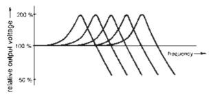
Fig. 5. Changing the frequency response with different external capacitors parallel to a pickup coil
