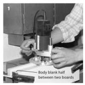
With appropriate jigs routers can also be used for jointing or planing. The following examples will illustrate how versatile routers are and how they can make buying a jointer or thickness planer unnecessary. Quite commonly the width of work that can be accomodated by most thickness planers used by hobby woodworkers is below what is required for preparing guitar bodies anyway.
