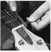
**Use of feeler gauges** You can avoid making nut slots too deep by placing feeler gauges of fret height under the nut file. This enables you to get the slot depth absolutely right.
