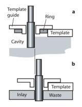
Flush-trimming cutter bits with shank-mounted ball bearing always have to be lowered deep enough for the ball bearing to be on the same level as the template (1). This is why the cutting depth cannot be below a certain minimum. If the cutter is too long, the template has to be made thicker. Such cutters are available in different cutting-edge lengths - the shortest one I know of has a 1/2" (12.7 mm)-long cutting edge.
