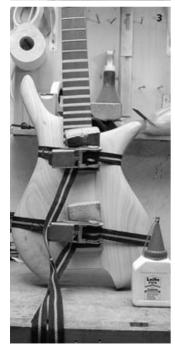
I marked the holes for the body wing dowels on the neck blank with metal dowel hole markers (1). Such markers are commercially available (at least in my part of the world). For drilling the holes into the neck blank I used the same set-up as on the body wings. If you want to use the drill press, note that the neck blank surfaces are slanted and that the table has to be tilted to get holes that are square to the surface. My "drill-stand method" automatically takes care of that.
