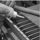
Pressing in the frets The method most commonly used nowadays by guitar manufacturing companies is to press the frets into the slots with special arbor presses and cauls whose bottom side is
