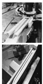
A **tablesaw can also be used** for cutting a straight truss rod channel. The desired width of the channel is obtained with a dado head or two or more cuts made next to each other with a normal sawblade.
