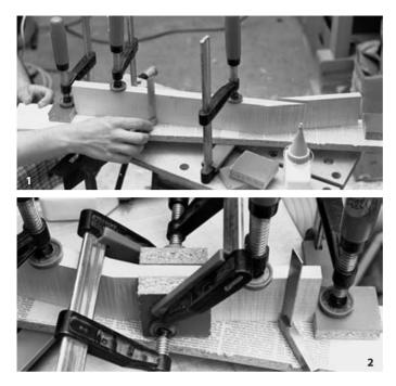
square to each other (1). Put some newspaper under the gluing area. Use a third clamp to hold a stop block on the lower end of the neck; this stop block is supposed to keep the neck blank from slipping away.
