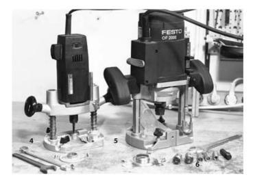
long as you make sure that the collet is *very well* tightened. Another drawback is the increased cutter vibration. Shank adapters are more of a makeshift and I would recommend that you to use a right-sized collet straight away.
