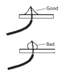
When carrying out soldering work on heat-sensitive semiconductor components such as diodes or integrated circuits (ICs) the soldering time must not exceed five seconds.
