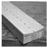
Making a radius-sanding block Long radius-sanding blocks for finish-sanding fingerboard surfaces are a great help. Necks with cylindrical fingerboard are moved over these blocks, which are fastened on the workbench in a lying position. As I am unfortunately not aware of any source of such (long) radius-sanding blocks, you will have to make them yourself.
