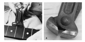
The frets should be installed as tight as possible in the slots to ensure a good sound transmission onto the fingerboard. Glue fills hollow spaces and thus improves the transmission of sound.
