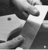
Then plane further chamfers as required to get the desired neck shape (1). Do not make the neck thinner at this stage or take anything off the sides of the fingerboard.
