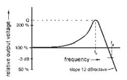
Fig. 4. Fundamental frequency response of a magnetic pickup. Position and height of the peak vary from type to type
