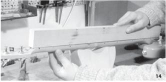
The frets can now be colored with a blue textmarker (12). Using a flat-surfaced sharpening stone, a commercially available fret-leveling file (13) or a home-made fret file (see drawing below) work all frets until metal reappears on them. An alternative would be to use a long straight-planed piece of wood (14), about 25mm (1") in width, onto the edge of which a strip of 120grit sandpaper is glued with spray glue. The piece of wood used should be slightly longer than the fingerboard.
