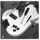
Fitting a headless unit Headless guitar tuning units are often fitted to the body at a small downward angle. For this you need an angled surface which can be made with a template fastened accordingly (1). Then test-fit the unit (2), fastening the head part at the end of the neck with two screws (3). The allen key demonstrates that ordinary strings without second ball-end can also be used.
