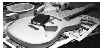
Before the final coat is sprayed on, the guitar should be sanded particularly well. The final coat is best sprayed with a mixture made up of equal parts of thinner and nitrocellulose lacquer. This will give a surface that is easy to rub afterwards.
