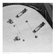
**Bridges mounted on two posts** Bridges mounted on two posts are positioned slightly out of right angles to the fingerboard center line to get the best intonation adjustment options possible. If the guitar is to have a separate tailpiece, fit it about 50mm (2") behind the bridge. How deep you will have to drill and what hole diameter will be required depends on the height-adjustment bolt bushings of both the bridge and the tailpiece.
