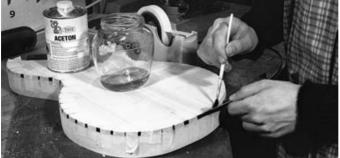
picture 7 you can see the rolled binding being used to check whether the router is correctly set. Rolling together the binding also makes it easy to sand away any bits of it that may be too high. The binding should protrude over the body only very slightly. Before starting work on the body practice on a piece of scrap wood. When everything is fine cut the rabbet(s) on the body (8).
