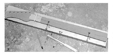
tuners fitted on one side) the neck center line will be either left or right of an imagined neck blank center line (**3**). Both the entire peghead and neck template have to fit on the neck blank. If you make a one-piece neck, also mark the center line and all other auxiliary lines on the back of the neck.
