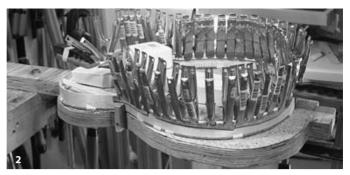
be the fastest way - with a bandsaw (1). Draw a line on the table of the saw to help you get equal distances (about 6 mm / 1/4") between the cuts. A depth stop ensures a small web (0.4 mm / 1/ 64") is left behind the cut. Finished strips, so called kerfed lining, can also be bought. As for which wood to use I would recommend mahogany, alder or spruce. The number of strips needed depends on the body circumference: twice its length will be needed.
