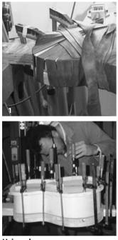
**Using clamps** If you use clamps for gluing on the back make a narrow guitar-shaped clamping caul like shown above.
