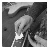
**Oiling the fingerboard surface** All fingerboards except lacquered maple ones require thorough cleaning and the application of a thin coat of fingerboard oil (available from guitarmakers' suppliers) or gun stock oil before the guitar parts are finally assembled.
