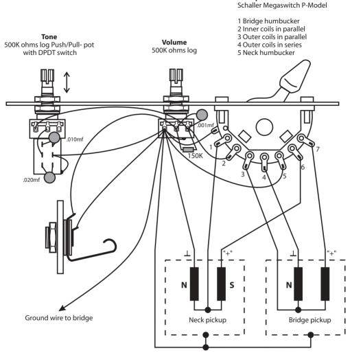
The outside coils of the pickups must have opposite magnetic polarity
