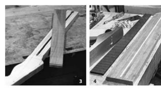
Drill two holes of the same diameter as the wire brads into the slot of the first fret and another two into the slot for the 15<sup>th</sup> fret. By drilling these holes the fingerboard is kept from splintering when driving in the nails (6). Have five strong clamps as well as all other bits and pieces needed ready at hand before you apply the glue; spread the glue thinly and evenly on the back of the fingerboard or within the fingerboard outline on the face of the neck (7).
