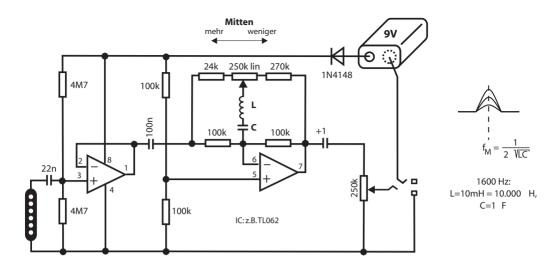
**State-variable filters** offer the maximum amount of freedom in shaping the tone of a pickup as they allow selecting and influencing of a specific frequency band with the frequency (control F) as well as the boost (control Q) infinitely variable between 0 and 12dB (quadrupling). Thus any tonal characteristic can be imitated and the properties of the passive pickup become less important.
