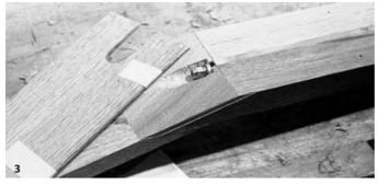
slanted at an angle of below 68 degrees to make it butt up against the nut. Also remember to cut out an opening for allowing access to the adjustment nut. Copy its outline on a piece of paper and transfer it onto the veneer. Only one layer of thin veneer must be glued onto necks without separate fingerboard (one-piece necks) and with angled-back head as otherwise the veneer would be in the way of the strings.
