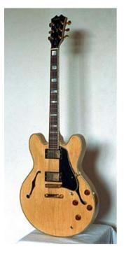
Semi-acoustic guitar Scale length: 24.75" (628.65mm) Neck: glued-in, angled head, maple, clear lacquer Fingerboard: rosewood, untreated Body:5mm-thick maple plywood, clear lacquer Greatest body width: 410mm (16.1") Body length: 490mm (19.3") Body depth: 45mm to 55mm (1<sup>3</sup>/<sub>4</sub>" to 2<sup>5</sup>/<sub>32</sub>")
