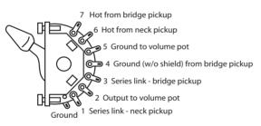
With Yamaha's four-pole five-position lever-action switch (12) a particularly high number of different combinations is made possible. Its wiring, however, is accordingly complex. This switch is available from *Stewart-MacDonald*. Because the wiring instructions that come with it are very detailed, I will not repeat them in this book. I would strongly recommend that you really only use such a switch if you consider the number of conventional pickup combinations not sufficient.
