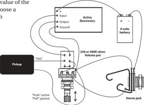
A totally independent mixing of pickup signals is only possible with an active system because here the volume controls do not interfere with each other and any combination of the signals of both pickups can be selected. The capacitors (dotted lines in the illustration below) are again used to lower the resonant frequencies of the pickups.
