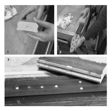
A cylindrical fingerboard will be produced if you consistently sand strictly parallel to the center line (b). For this purpose only may a radius-sanding block be used over the whole length of the fingerboard. Wooden or synthetic sanding blocks for the most common fingerboard radii are available via mail order from guitarmakers' suppliers (1).
