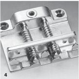
On systems where the tremolo is mounted so that it "floats" players used to resting their hand on the bridge in doing so often unintentionally operate the tremolo. To prevent this from happening, a mechanical lock (sometimes called "Black box") was invented which only unlocks the tremolo when a certain amount of pressure is exerted on the arm. Such systems are hinged between the tremolo block and the springs.
