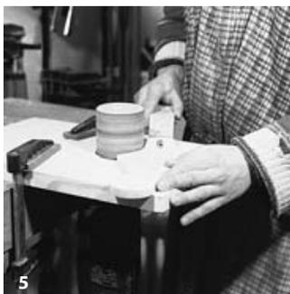
Finish off by smoothing and sanding the head to shape (5,6). Be patient, watch out for uneven curves, and make corrections if necessary.
