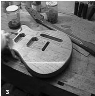
**Finishing the body and the neck with Danish Oil (2)** saves time, gives good results and can therefore only be recommended. Danish Oil is an oil-varnish blend. It cures to a satin sheen and is much more protective than boiled linseed oil while being just as
