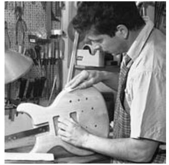
Before the final coat is sprayed on, the guitar should be sanded particularly well. The final coat is best sprayed with a mixture made up of equal parts of thinner and nitrocellulose lacquer. This will give a surface that is easy to rub afterwards.
