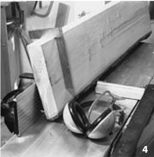
Cut a straight edge on the tablesaw (3). Since in this state the plank cannot be guided along the rip fence of the tablesaw, I placed it on a rectangular jig. The guard was removed only for taking the picture.
