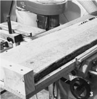
Start by planing one of the surfaces flat (2). Move the plank over the jointer, using a push stick for pushing it. The shape of the push stick does not really matter; it can be rounded off and given a more hand-friendly shape than the one in the picture. When planing hardwood not more than 3mm ( $\frac{1}{8}$ " should be planed off in one pass and several passes may be required until the surface is flat. If the plank is too wide for the jointer, reduce its width with a tablesaw (see below).
