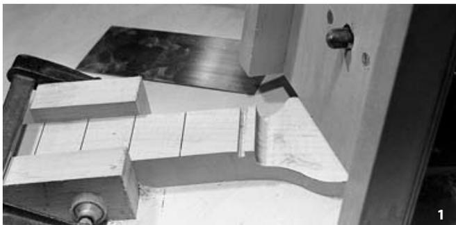
The curve towards the nut can also be made with a cove bit. In picture 1 you can see me using a small-radius cove bit; I used it only because I didn't have a bigger one. A greater radius is preferable, though, not only because it looks better, but also because it gives better stability. The picture is only to illustrate the basic idea. Make sure to set the stop blocks very accurately.
