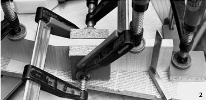
square to each other (1). Put some newspaper under the gluing area. Use a third clamp to hold a stop block on the lower end of the neck; this stop block is supposed to keep the neck blank from slipping away.
