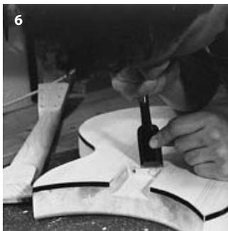
**If you make the angle on the neck pocket in the body**, the template has to be placed at the appropriate angle. You can use the same "three-boards"-technique that was used for aligning the neck and cutting out the neck pocket, but you can obviously also make one sufficiently large and tight-fitting template from one piece (3). The angle can be made greater or smaller by placing a wooden shim across the rear end of the template and
