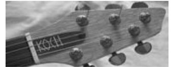
When tuners are fitted on both sides of the peghead a straight string line can only be achieved by mounting the tuner pairs successively closer to each other towards the end of the peghead. Unfortunately, the tuners traditionally used do not allow a symmetrical layout of the two top tuners as the distance between the two middle strings is too small. The solution is to use a staggered tuner layout (3), which inevitably makes the peghead asymmetrical.
