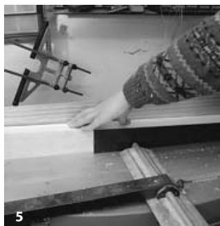
The body offset is best made with a jointer that allows lowering the infeed table by the seven millimeters that are required. Since I didn't have access to such a jointer, I routed the body part down to the right thickness using a big surface trim bit as shown in picture 6.
