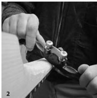
Before I glued on the body wings I marked their upper ends on the neck blank and shaped as much of the neck profile as possible (2). Rough-shaping the body-neck transition is also easier without the wings glued on.
